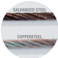
Comparison of materials after 10 years stuck in the ground.
